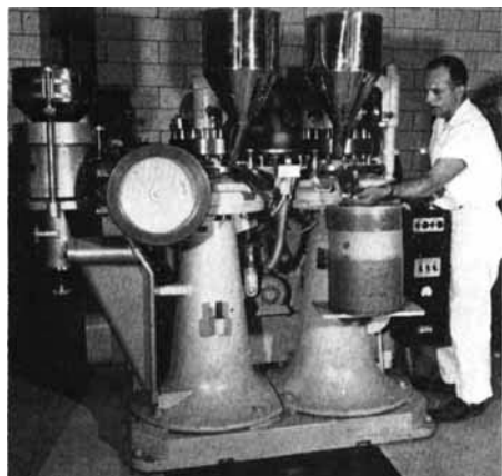
Fig. 1.—Photograph illustrating the Manesty Dry-Cota machine.
